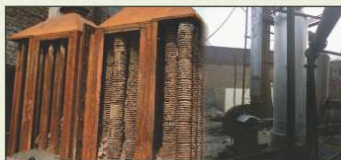
Conventional Recuperator shell & Tube Type installed under ground
